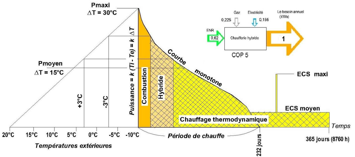
The figure above shows how the hybrid boiler adapts its power and satisfies the thermal need during the heating period. This by providing a heating power substantially proportional to the temperature difference  $\Delta T$  that should reign in the living rooms and the outside temperature.
