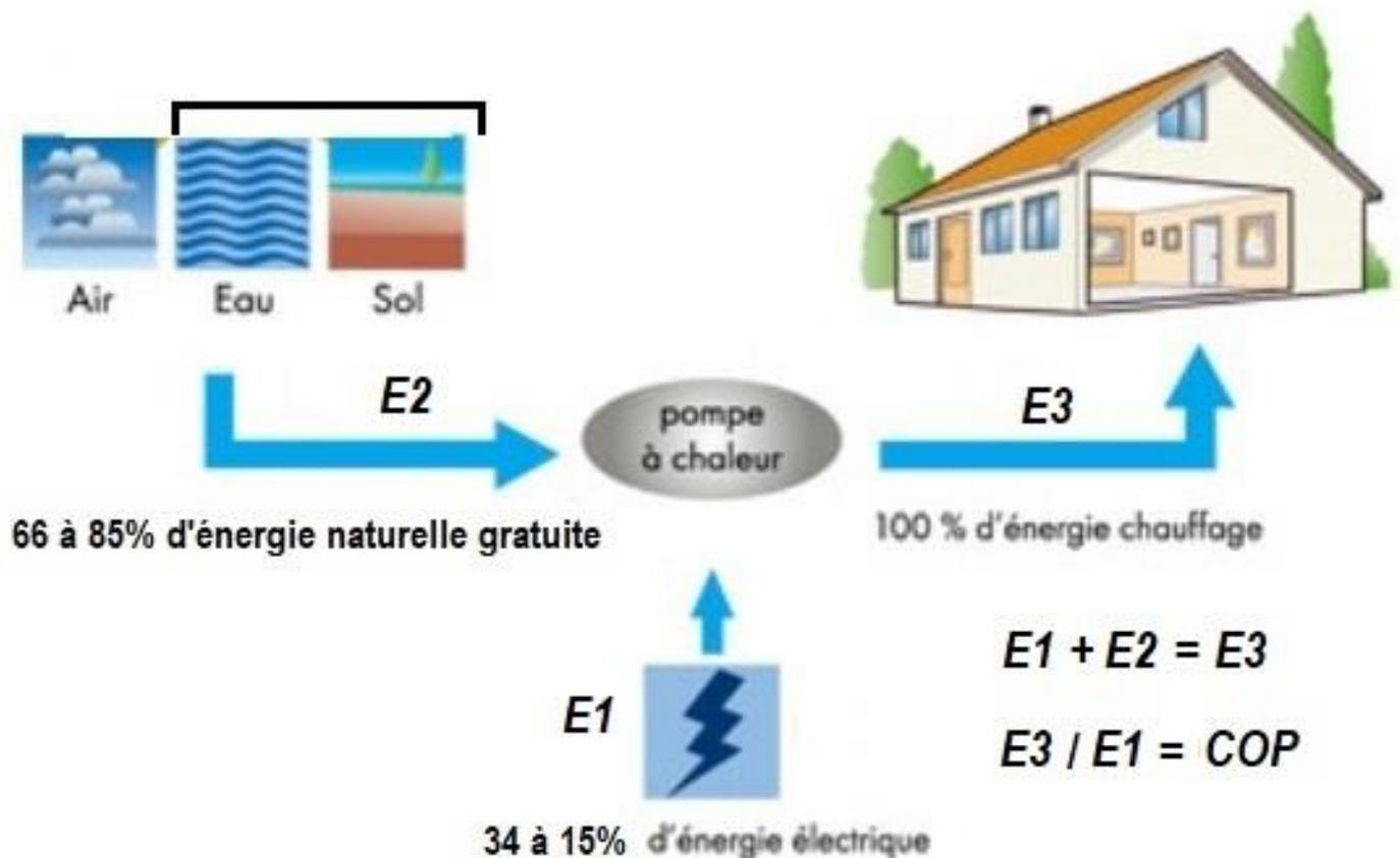
It is by comparing between them the two energies it receives, the one that is taken from the water and the one that one pays that one realizes the energy potential of the heat pump. It is important to know that the free energy from the natural environment can be 2 to 4 times or even 6 times greater than the electric power that drives the compressor. There has been a significant
