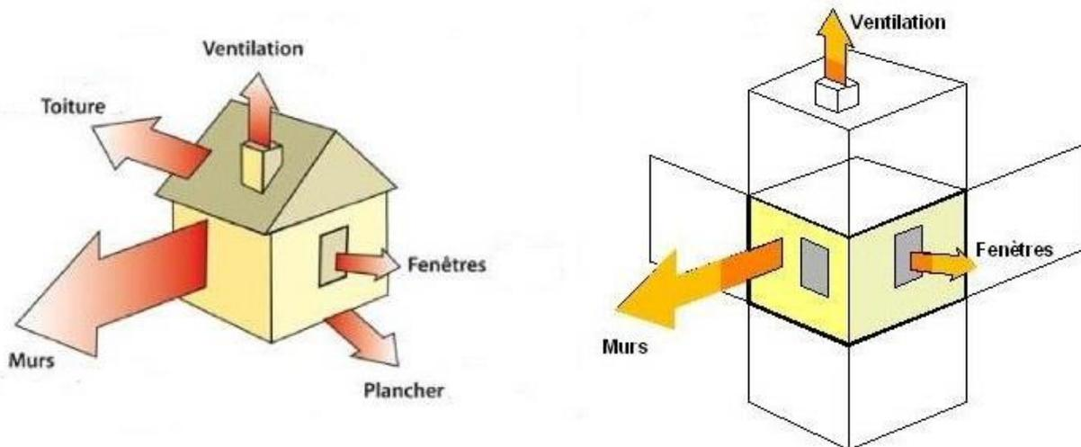
**Figure 8** A two-exposure apartment on the middle floors with tier edper neighbours is subject to significantly lower energy consumption than a detached house of the same living space. This is for equivalent loss coefficients(see [P144](#))and buildings located in an equivalent temperature zone (see [P278](#))
