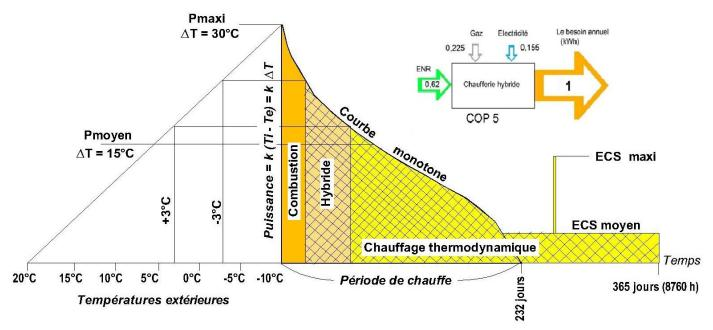
The figure above shows how the hybrid boiler adapts its power and satisfies the thermal need during the heating period. This by providing a heating power substantially proportional to the temperature difference  $\Delta T$  that should reign in the living rooms and the outside temperature.
