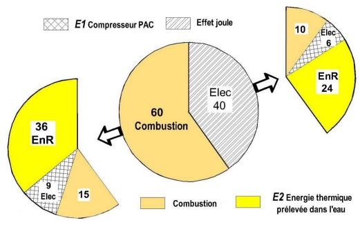
Minimum performance in heat pump mode by taking from the water
