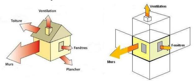
**Figure 8** A two-exposure apartment on the middle floors with tier edper neighbours is subject to significantly lower energy consumption than a detached house of the same living space. This is for equivalent loss coefficients ( $\sec P144$ ) and buildings located in an equivalent temperature zone (see P278)
