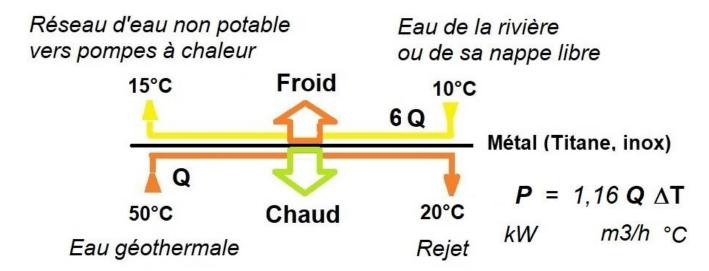
Water-specific heat 1.16 kWh/degree per m3
