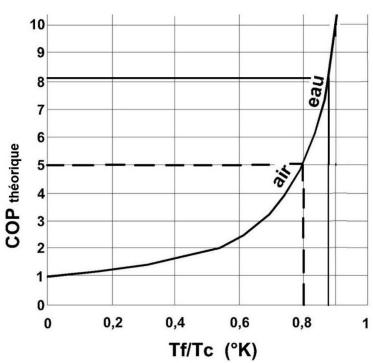
The value of exchanging renewable thermal energy on water rather than air is measured here. This is because the amount of electrical energy required to heat the habitat is about twice as low as with air at the same temperature at the hot spring or what amounts to the same temperature in the radiators Hydraulic.
